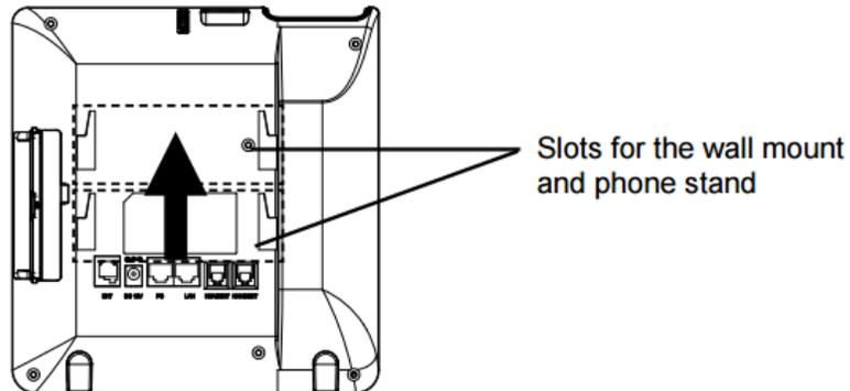
Figure 2: Slots for the wall mount and phone stand on the GXV3240.
