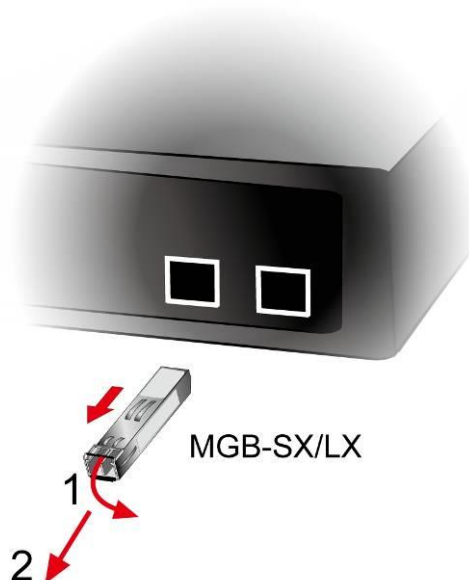
Figure 2-1-2d How to Pull Out the SFP Transceiver
