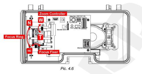
For easy camera lens setting, use the scheme attached on the inside of the camera cover (*Pic. 4.6*).
